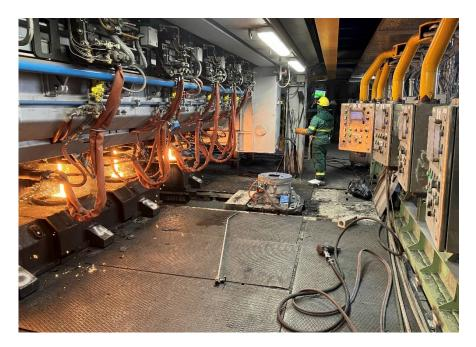
Retractable oscillators from Primetals Technologies allow for the exchange of molds during casting sequences, resulting in increased productivity.
