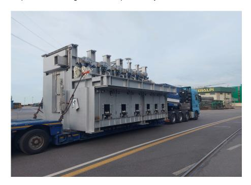
Primetals Technologies designed the 6-strand billet caster bow in one piece to ensure a minimized shutdown period.
