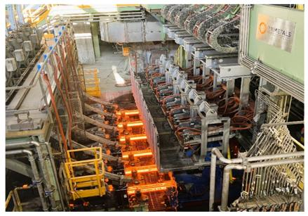
The revamped 6-strand billet caster from Primetals Technologies at Italian steel producer Feralpi's site in Lonato del Garda, Italy.
