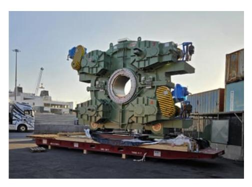
The new tilting drive from Primetals Technologies on its way to South Korea as one 110-ton piece.
