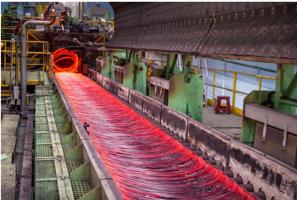
Hot wire rod coil exiting Morgan High-Speed Laying Head and cooling as it moves down the Morgan Stelmor Cooling Conveyor
