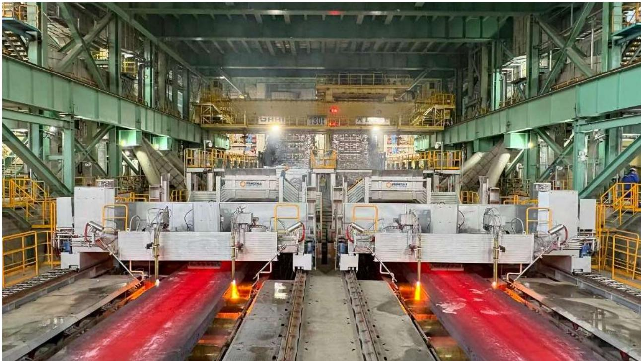
Baosteel's new ultra-thick slab caster from Primetals Technologies can produce slabs up to 460 millimeters thick.
