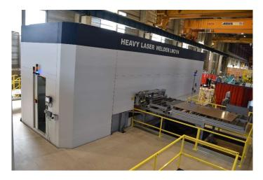
The advanced laser welding machine (LBW) to be applied in the pickling line modernization. Shown here is an identical implementation to the one for Toyo Kohan.
