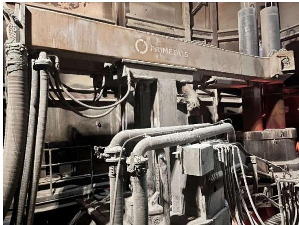
New electrode arms from Primetals Technologies boost power output and reduces energy consumption at Tonghua Iron and Steel.
