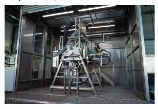
The new heat transfer test facility from Primetals Technologies allows for optimization of industrial cooling systems.
