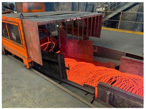
Close-up of 8-millimeter wire rod exiting laying head onto the cooling conveyor at Stahl Gerlafingen's new wire rod mill, supplied by Primetals Technologies.
