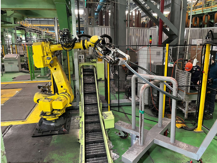
TrimRob autonomous coil trimming and sampling robot from Primetals Technologies and Polytec
