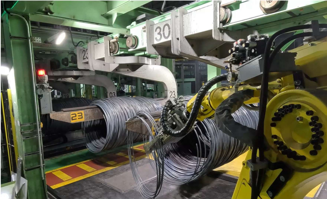
TrimRob autonomous coil trimming and sampling robot from Primetals Technologies.
