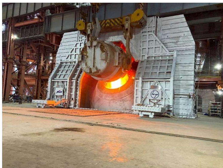
The first charging at JVML's LD converter (BOF) "H", supplied by Primetals Technologies.
